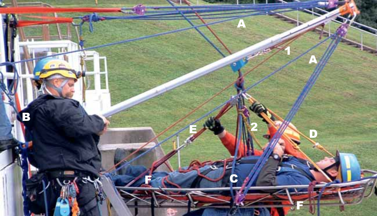
Rescue practitioners working over difficult spillway in Indianapolis during 2006 Ropes That Rescue workshop. Gin pole is held by three AZTEKs used as adjustable guys and one AZTEK "dynamic directional" (see 1). Rescue attendant is hanging from AZTEK "set of fours". Also in photo, short leg purcell used as a safety lanyard for rescuer (see 2).
